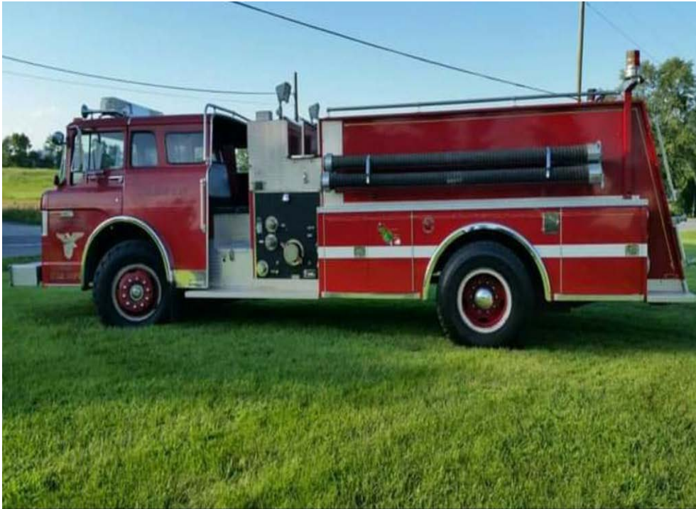
1982 Ford C800, Body by Pierce 1000 GPM - Top mount Pump Panel
